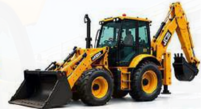
BACKHOE LOADER 3CX / CASE 570T / CAT 426F2 JCB / CASE / CAT
